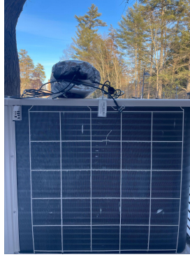
Figure 5: (Left) Coil side of the ODU showing the temperature sensor directly on the fins of the unit, also on top is the insulated packaging we designed for the LabQuest2 to keep it from malfunctioning in the cold weather
