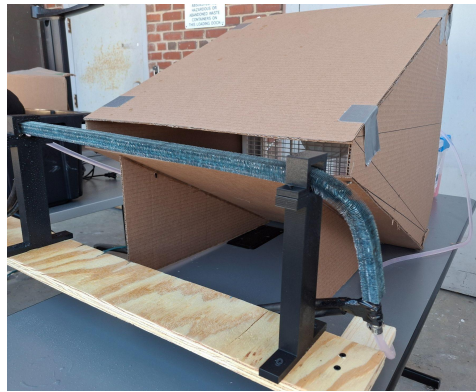
Figure 2: Image of coil testing set up on an ASHP coil with PETD integration (as a peak on what is to come with our PETD and ASHP integration)
