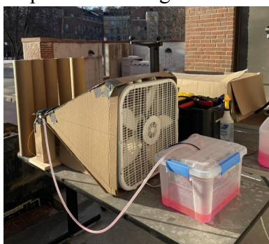
Figure 24: The full prototype testing setup in operation outside. The fluid loop is pumping RV antifreeze through the coil, while the fan is blowing onto the coil on the left. The transformer is inside the bin to maintain some degree of safety. The cardboard tubes were put in place to provide shade.
