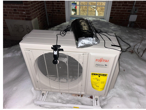
Figure 5: (Left) Coil side of the ODU showing the temperature sensor directly on the fins of the unit, also on top is the insulated packaging we designed for the LabQuest2 to keep it from malfunctioning in the cold weather
